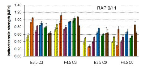
> As expected, mixtures with cement show higher values of strength for the different curing procedures, with exceptions when accelerated curing using relatively high temperature (3 days @ 50°C) is applied.
