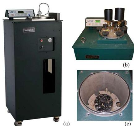
Figure 4-2: Moisture induced sensitivity tester or MIST
