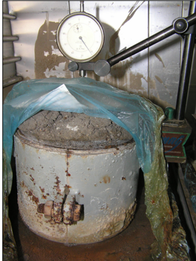
Fig. 10: View of a sample compacted by 100 % Standard Proctor energy at the temperature of 75 °C after 65 days.
