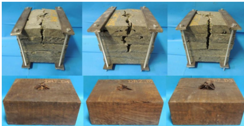
Fig. 8: The specimens made of recycled plastic and of oak wood after conducting the screw spike pullout test.
