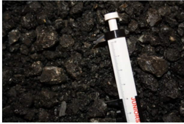
Fig. 2: Multiple aged and crushed RAP.
